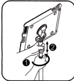
To raise or lower the Gripbase Podium, loosen the collar and raise.
