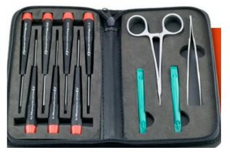
The included tools are these: 2 slotted screwdrivers, 2 Phillips head screwdrivers and 3 Torx drivers. This latter tool is for those fasteners that have a hole with inside flanges. There are 2 special-purpose tools which the Company calls "spudgers," nylon pry tools for opening those difficult to open but easy to scratch cases. Lastly, there are two grippers that are so useful for small pieces that can otherwise slip down into the works.
