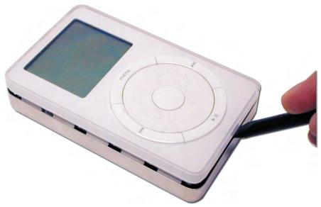
Work the nylon tool in from the bottom of the unit once you have the left side released. There are 2 clips on the bottom to unlock. Be careful to not put pressure on the back of the case and accidentally close the top left side where you began the process.
