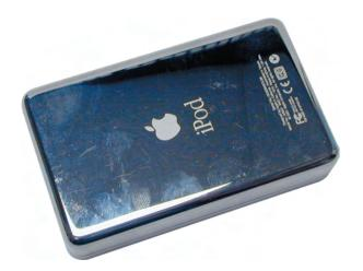
Slide the iPod back cover onto the front shell and gently press toward the front to snap it back on.
