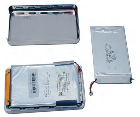
Insert the replacement high-capacity battery onto the logic board socket, it will only plug in one direction. Then, place the battery back onto the adhesive strips, centering it's position on the iPod as shown. Tuck the wires in neatly to the top of the battery, making sure they do not protrude from the inside of the case.
