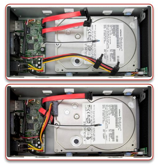
Set your hard drive into the chassis as shown above, sliding the drive as far forward as it will go. Lift the rear of the drive up and plug the bottom multicolored power cable and the inside red SATA cable into the hard drive. Place the white and black thermal probe wire above the drive.
