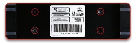
Again, lay the Newer Technology Guardian MAXimus onto it's side and insert the 4 black Phillips screws (2 you removed to start this process, and 2 from the bag) through the outer shell into the inner chassis, fully fastening the Newer Technology Guardian MAXimus together and completing the assembly process.
