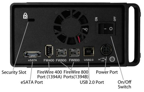
Turn the Newer Technology Guardian MAXimus so you can see the rear port as shown above. First, make sure that the power switch is off. Then, connect the power cable to the back of the Guardian MAXimus. Finally, you need choose which interface you want to use to connect to your computer.
