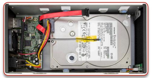
Turn the chassis back over so you can see the drive inside. Take the included yellow kapton tape and attach the black and white thermal probe as close to the center of the hard drive spindles as possible. Do not tape over the blue thermal probe lead, but rather tape the wire down to the top of the drive as shown.
