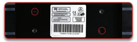
Turn the Newer Technology Guardian MAXimus onto it's side and remove the 2 screws that are fastening the outer shell to the inner chassis. Removing the 2 screws will release the inner chassis. Slide the inner chassis out of the shell from the back to the front.
