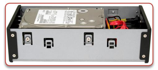
Once the cables are installed, look at the side of the drive chassis and align the screw holes in the sides of the hard drives up and fasten the same collared screws that you used on the bottom drive through the silicone rubber grommets and attach one side of the hard drive into the chassis. Repeat on the opposite side of the chassis.
