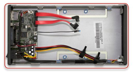
Once you have removed the inner chassis, look into the chassis and you will see the cables, and screw holes that you will be using in future steps. Do not disconnect any cables, or change any jumper settings. The Newer Technology Guardian MAXimus is preconfigured as a RAID-1 Mirror and does not require any changes.
