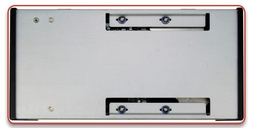
Here you see the bottom of the Newer Technology Guardian MAXimus chassis with 4 screws inserted into the bottom hard drive mechanism. Line the 4 screw holes up and insert the collared screws that are included with the kit through the silicone rubber grommets and tighten only partially until all 4 screws are inserted fully.
