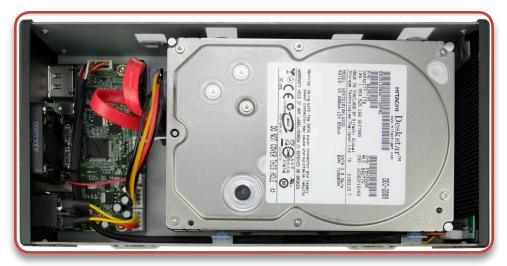
Gently set the 2nd hard drive on top of the lower drive that's already installed into the chassis and once again, plug in the multicolored power cable and red SATA cable into the drive. This drive is easier to install.
