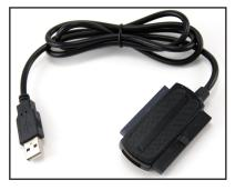
Start by locating the Universal Drive Adapter. You will need this to connect any type of drive mechanism to your computer. Notice that on one end there is a USB 2.0 connector, and the other end has three separate connectors on it, a full size 40 Pin ATA connector for 3.5" ATA drives / 5.25" ATAPI devices, a mini 44 Pin ATA connector for 2.5" drives, and there is also a Serial ATA (SATA I or SATA II) connector molded into the very end of the adapter.
