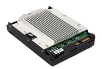
**2.** Place your SATA drive onto the mounting bracket as shown. The connecting cables need to be positioned to the left, with the opening in the drive bracket to the top. Once inserted properly into the bracket, insert the 4 Phillips screws to fasten it securely.
