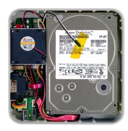
**3.** Place the drive and bracket inside the Newer Technology miniStack v3 enclosure, routing the power and SATA cables to avoid pinching them. The SATA cable will need to be tucked around the corner of the hard drive at an angle once it's set into the drive enclosure.
