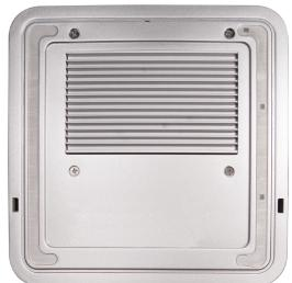
**1.** Begin by removing the 4 Phillips screws from the bottom of the Newer Technology miniStack v3 enclosure. Remove the aluminum drive carrier from inside of the Newer Technology miniStack v3 enclosure.
