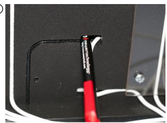
Using a retractable pen (a flat tool that you can push with, and not cut the cable is all that's required), gently push on each side of the dock connector to release it from the dock cable slot. Once you press it out of the slot, the pen will slide into the GripStand Station housing.
