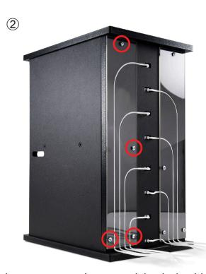
To remove a 30-pin dock cable, turn the GripStand Station so that you can see the rear and the dock cable channels. Determine which cable you want to remove (in this scenario, the second cable from the bottom will be replaced). Unscrew the four Phillips screws that secure the clear plastic cable cover (circled in red in step ②), and remove the plastic cover.
