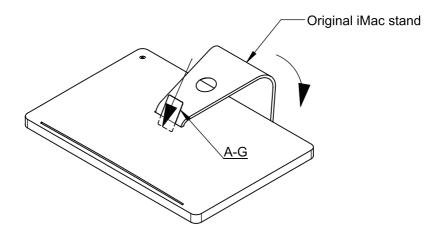
Step 2: With the card in the slot, lower the stand as far down as it can go; you will see screws where the stand connects to the iMac. Separate the stand from the iMac by using the Torx tool (A-E), as shown below. Set the original M3 screws aside — there are 8 in total.
