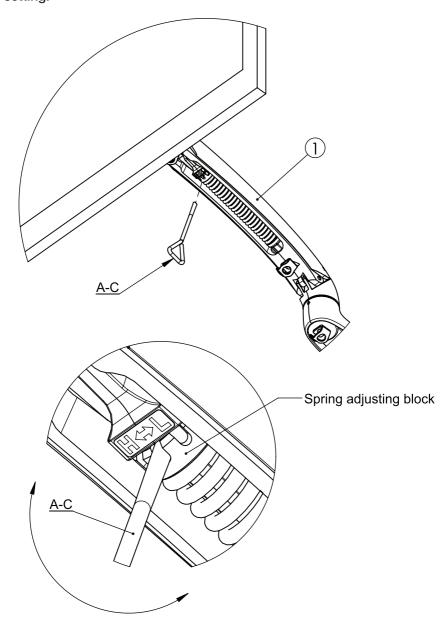
Note: how far the display can be extended is dependent upon the tension in the adjustable spring described on the previous page.
