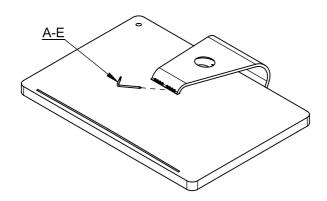
Step 3: Use the Torx tool (A-E) to fasten the Mounting Plate to the iMac as shown, using the M3 screws that were removed in the previous step.
