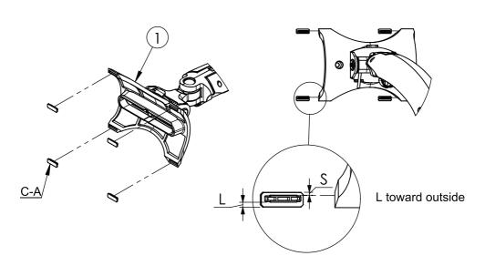
Step 5: Using the A-D wrench and the A-F screws, fasten the Display Arm onto the Mounting Plate as shown below.
