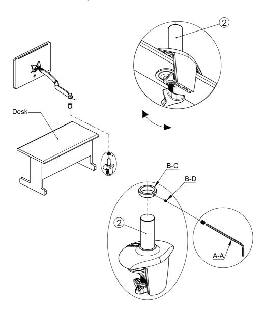
Step 8: Install the Adjustable Arm Sleeve (B-B) into the Display Arm, as shown below. Note the sleeve gap location.
