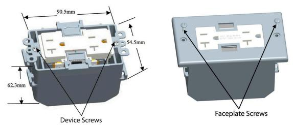
① Turn the power back on to the receptacle at the circuit breaker or fuse panel. Test the Power2U receptacle (125V) power outlets and the 5.2V USB outlets to verify proper operation. The USB outlets are only powered when the safety switch cover is open and a USB cable is plugged in. If a USB port does not work when installed, please visit http://www.newertech.com/p2u-install for troubleshooting tips and suggestions.
