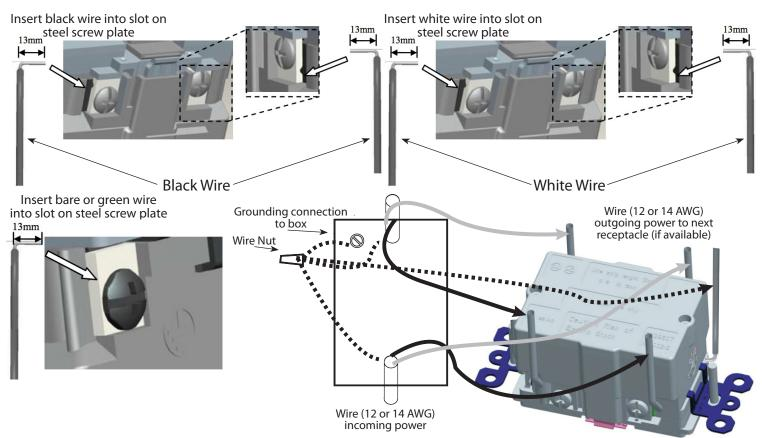
③ Fold the wires into the electrical box, keeping the bare ground wire away from the HOT (brass) and Neutral (silver) terminals. Screw the Power2U into the electrical box. Screw the faceplate into the Power2U.
