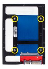
There are eight Phillips head screws included. Use the four fine-threaded screws to fasten the AdaptaDrive to the SATA drive.
