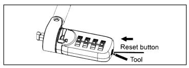
**Step 3** - While holding in the reset button, set a new four digit combination, making sure to align the numbers with the combination notching line as you did in Step 1.
