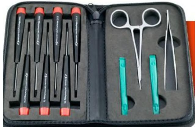
The included tools are these: 2 slotted screwdrivers, 2 Phillips head screwdrivers and 3 Torx drivers. This latter tool is for those fasteners that have a hole with inside flanges. There are 2 special-purpose tools which the Company calls "spudgers," nylon pry tools for opening those difficult to open but easy to scratch cases. Lastly, there are two grippers that are so useful for small pieces that can otherwise slip down into the works.
