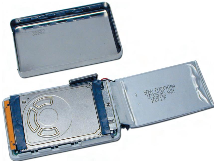
Gently work the battery from the iPod, there are 2 black adhesive strips on the top and bottom of the battery to release. If they stick to the battery, simply peel them off and reapply them to the top of the hard drive as shown here. It may take some force, and you may use the nylon tool to pry the battery off, using gentle force.
