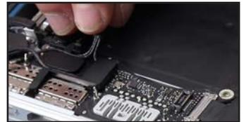
16. Next, lift up the latching handle on the lower I/O board cable.
