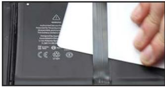
46. Slide the cable from the ZIF connector that was opened in Step 44, then set the cable aside.
