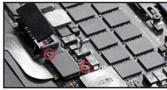
98. Align the battery connector with its socket and press it down, snapping into place.
