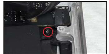
10. For 2013 and 2014 models, there are four additional screws to be removed, two on each side of the center battery cells.
