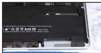
30. Set the right speaker assembly back into place, making sure that its wire is routed under the metal screw post. Secure the speaker with its three screws, making sure to affix each screw in the same location it was removed from in Step 7. NOTE: If you're not using a 2015 model, skip ahead to Step 32.
