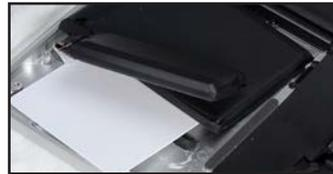
15. Using the syringe apply about a quarter of a milliliter of adhesive remover under the outer battery cell on the opposite corner and let it sit for about a minute.
