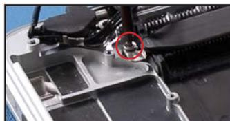
37. Lift the bar of the microphone's ZIF socket and slide the cable free.
