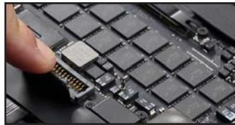
6. Remove the two Torx T5 screws shown, then remove the trackpad connector cover (below-right).
