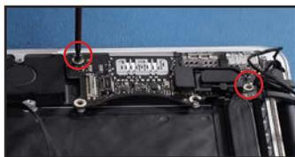
69. Attach the lower I/O cable by sliding it into its socket and using the handle to latch it into place.
