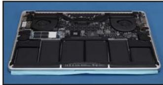
5. Disconnect the battery by pulling back the cover (red), then lift the connector upward using the included nylon pry tool or a fingernail.
