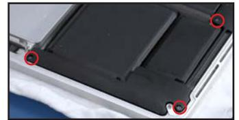
12. Lift the speaker assembly up, and rotate it so that it sits out of the way.
