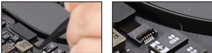
31. Following the same process as in Step 19, lift the fan out of the chassis, then peel the cable up from the logic board if necessary and remove it from its socket.
