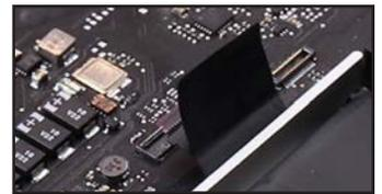
29. Detach the trackpad connector by lifting it off the logic board.
