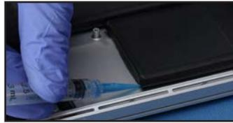
48. Work one of the plastic cards underneath the battery cell, slicing through the weakened adhesive strips until it detaches.
