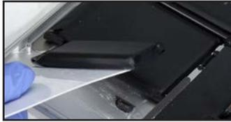
13. Hold the first cell out of the way, then repeat the process from Step 12 on the neighboring cell. Again, try to use a little adhesive remover as possible.
