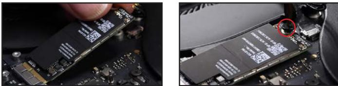
86. Attach the antenna cables by lining up their connectors and snapping them down onto the card.
