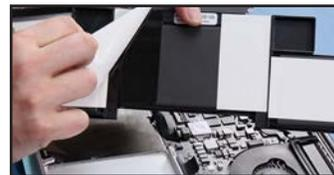
90. Align the battery connector (red) with its socket (yellow); press down.
