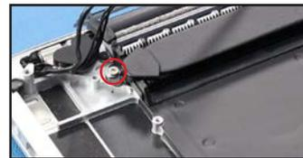
38. There is a corresponding silver screw near the back-left corner of the chassis, hidden underneath a rubber cover. Lift the cover off the screw using your fingers or the nylon pry tool, then remove the screw.
