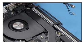
17. Remove the three Torx T5 fan screws highlighted below. Note the location of each screw before setting them aside; each is a different length and will need to be re-affixed in the same location later.
