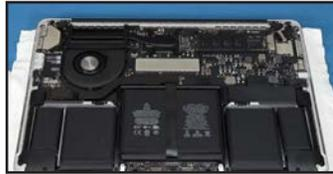
5. Disconnect the battery from the logic board by lifting the connector until it detaches. Afterward, if you're not using a 2015 model, skip ahead to Step 7.
