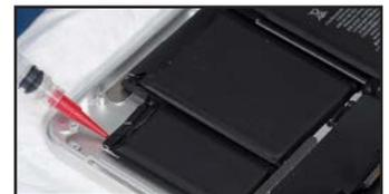
12. Starting at the corner, work one of the plastic cards underneath the battery cell, slicing through the adhesive strips until the cell detaches. If you need to apply extra adhesive remover, try to use as little as possible.
