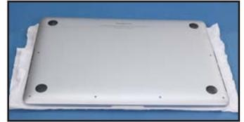
42. Re-affix the two shorter center screws along the hinge edge first. These screws were originally removed in Step 2.
