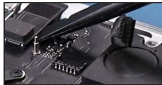
22. Lift the latch on the display data cable.
