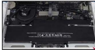
27. Re-affix the screw near the battery connector that helps keep the battery in place.
