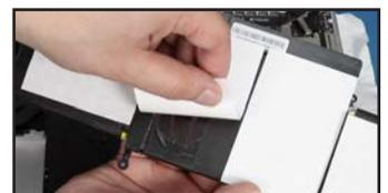
26. Set the battery unit in place, making sure it lays flat.
