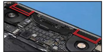
91. Peel off the four white paper adhesive covers on the back of the new battery.
