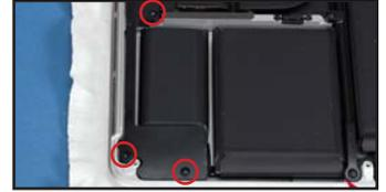
8. Lift the left and right speaker assemblies out of their channels and lay them back on the logic board. Do not put excessive tension on the wires as you may damage them. Note: the left speaker is shown in the top row.
