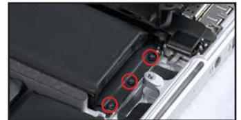
14. Remove the three Torx T5 screws which hold the right speaker in place (opposite corner). Note each screw's location. They are different lengths and need to be re-affixed in the same locations later.
