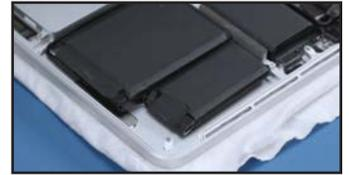
13. Remove the three Torx T5 screws securing the top part of the battery.
