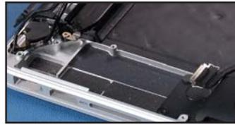
20. Peel the rubber cover off the left fan and set it back, out of the way.
