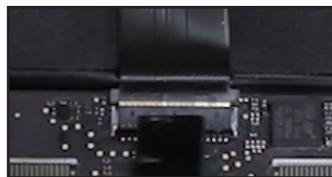
32. Reattach the battery by lining up its connector and pushing it into place.
