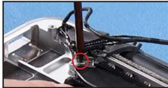
64. Re-affix the smallest logic board screw in the location shown.
