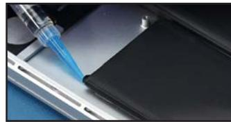
48. Starting at a corner, work one of the plastic cards underneath the battery cell, slicing through the adhesive strips until it detaches. You can use more adhesive remove if you need to, but try and use as little as possible.
