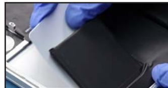
49. Holding the first cell out of the way, repeat the process on the neighboring cell. Again, try to use a little adhesive remover as possible.
