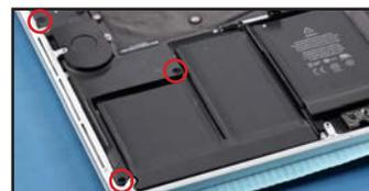
42. Lift the speaker up and out of the chassis.
