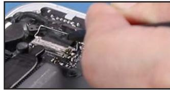
23. Slide the cable out of its socket.
