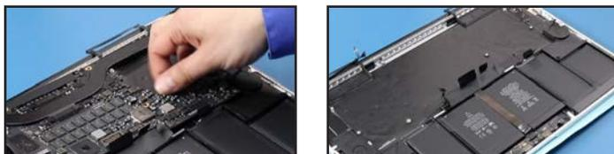
41. Remove the three screws shown at right, that hold the right speaker assembly in place.
