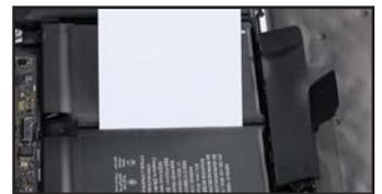
56. Apply about a quarter milliliter of adhesive remover along the base of the card, so it can run under the cell. Allow it to sit for a minute.
