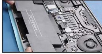
92. Replace the two battery board retaining screws, and then press down lightly on the battery to make sure it adheres to the case.
