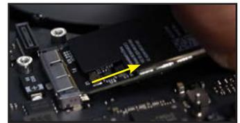
16. Slide the camera cable connector out of its socket, then lift the bundle of cables up and off the fan, and out from the cable guide on the other side.
