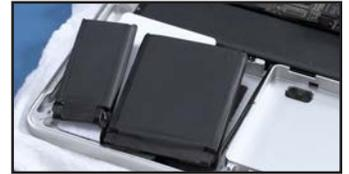
25. Lift the battery up and out of the chassis, then set it aside.
