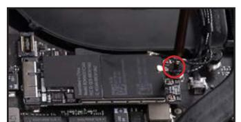
75. Attach the antenna cables by lining up their connectors and snapping them down into place.
