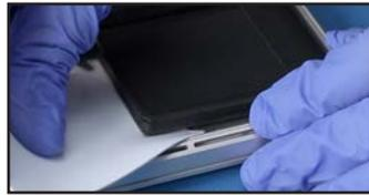
49. Hold the first cell out of the way, then repeat the process from Steps 47-48 on the neighboring cell.
