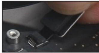
20. Lift up the latch on the lower I/O board connector.
