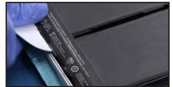
55. Once all the cells have been detached, you should be able to lift the whole battery up and out of the chassis.
