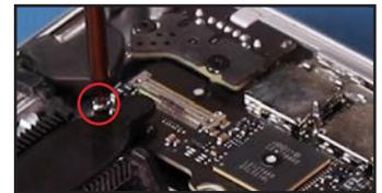
28. Pull back the label covering the keyboard connector (red), then use the nylon pry tool to lift the bar, disconnecting the cable; slide the cable free.
