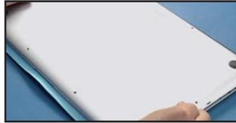
100. Re-affix the two center screws along the hinge edge which you removed in Step 2.
