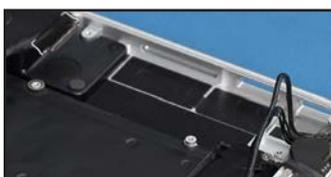
23. Lift the keyboard backlight cable connector from its socket using the nylon pry tool.
