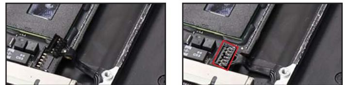
78. Snap the keyboard backlight cable into place.
