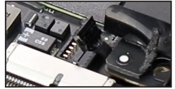
25. Peel back the label covering the keyboard connector cable.
