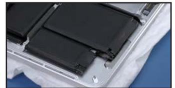
16. Remove the three Torx T5 screws securing the top part of the battery (opposite side).
