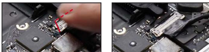
86. Slide the left fan cable into its ZIF socket and latch it down, using the same methods shown in Step 70.
