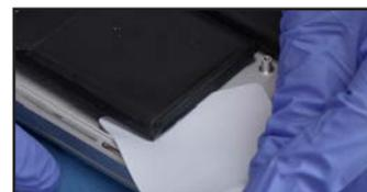
45. Hold the first cell out of the way, then repeat the process on the neighboring cell. Try to use a little adhesive remover as possible.
