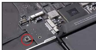
34. Next remove the two screws near the center of the hinge edge.
