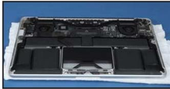
5. To disconnect the battery, peel back the label shown at right in order to access the Torx T6 screws holding the battery board in place.
