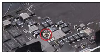
36. Last, remove the silver screw near the back-right corner of the chassis.
