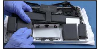
26. Remove the remaining adhesive from the battery compartment so that the new one has a clean surface to adhere to. To do this, use a few drops of the adhesive remover and the nylon pry tool to scrape it up, then peel and remove the rest with your fingers.
