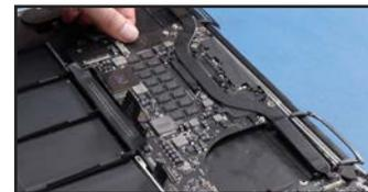
41. Remove the three right speaker assembly screws (shown in red) then lift it up and out of the chassis.
