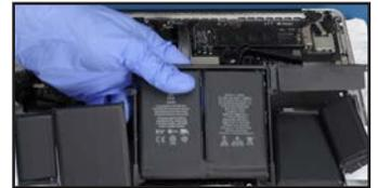
23. Remove the remaining adhesive from the battery compartment so that the new one has a clean surface to adhere to. To do this, use a few drops of the adhesive remover and the nylon pry tool to scrape it up, then peel and remove the rest with your fingers.
