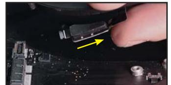
15. To remove the I/O board, first remove the camera and antenna cables from their guides.
