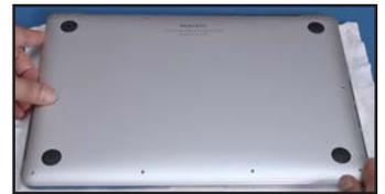
34. Re-affix the two shorter center screws along the hinge edge first. These screws were originally removed in Step 2.
