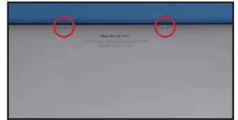
43. Re-affix the remaining 8 screws around the edges of the cover.
