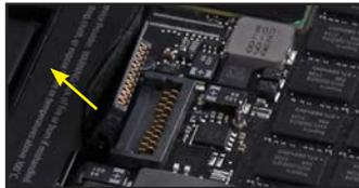
6. Remove the SSD retaining screw, then slide drive out of its socket.
