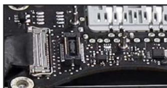
70. Insert the right fan cable connector (orange) into its ZIF socket (red) and then slide the latch (blue) down with your finger or nylon pry tool.
