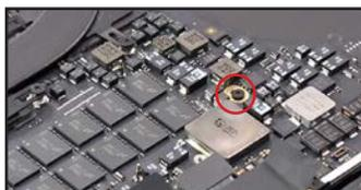
36. Next remove the two screws near the hinge edge.
