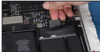
6. Disconnect the trackpad by first lifting the latch on its ZIF connector...
