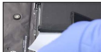
50. Once both cells are loose, use one of the plastic cards to hold them off the surface of the chassis so they don't accidentally re-adhere to it.
