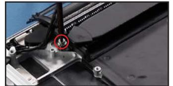
68. Re-affix the screws you removed in Step 36 along the hinge edge.
