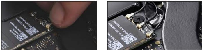
87. Align the SSD card with its socket, slide it into place, and secure it with the screw you removed in Step 10.
