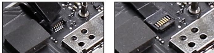
85. Slide the display data cable into its socket (top row) and then when the latch is raised (red, bottom-left), push it down to secure the connection.
