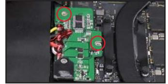
40. Whether it came separately or attached to the battery, you'll now need to peel any paper backing off of the PCB cover label and set it into place so that it is covering the battery connection and wires.
