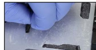
24. Wipe up any extra adhesive remover and let the computer sit for about half an hour to ensure any residual adhesive remover has evaporated.
