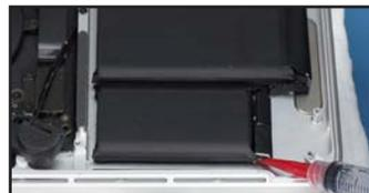
16. Work one of the plastic cards underneath the battery cell, slicing through the weakened adhesive strips until it detaches.
