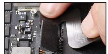
97. Reseat the trackpad's connector cover and secure it with the two screws you removed in Step 6.
