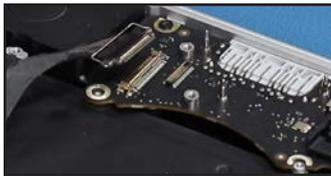
22. Remove the two Torx T5 screws (highlighted) holding the I/O board in place, then lift the I/O board using the nylon pry tool so you can remove the board itself.
