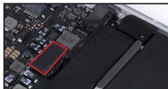
33. Set the cover back in place, making sure all edges sit flush with the computer's chassis.
