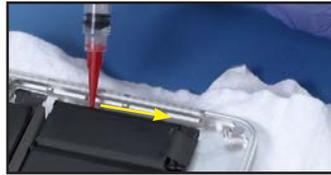
18. Then, work one of the plastic cards underneath the battery cell...
