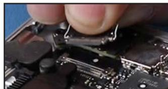
24. Lift the latch for the fan cable's ZIF connector. Minimal force is required.
