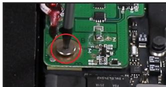
38. Re-affix the cover for the flat-headed screw, then secure it with the silver barrel screw.
