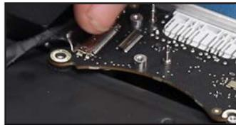
21. Loosen the connector's cable (top-left) then slide the connector out of its socket (top-right).
