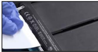
53. Apply about a quarter milliliter of adhesive remover along the base of the exposed card. Allow it to sit for a minute.
