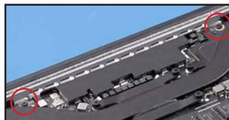
35. Then remove the screw near the memory.
