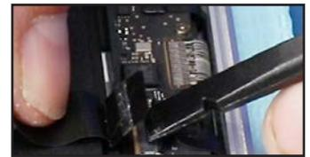
96. Line up the connector on the other end with its socket on the logic board and snap the two together. Re-attach the cable to the new battery using any residual adhesive that may be left on the cable.
