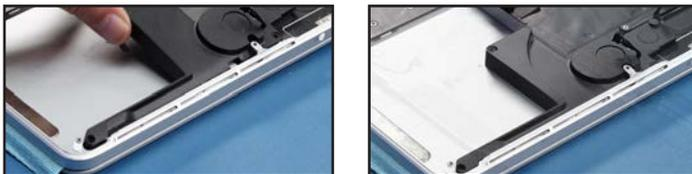
64. Set the logic board back into place, making sure it sits flat within the chassis and that no cables get trapped underneath.
