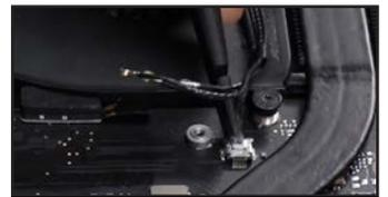
74. Align the wireless card with its socket, slide it into place, and secure it with the screw you removed in Step 6.
