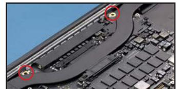
69. Re-affix the screw you removed in Step 35 near the memory.
