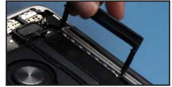
14. Unsnap the antenna cable connectors (red) from the wireless card by carefully lifting them from the card with the nylon probe tool.
