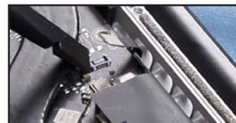
39. Remove the two Torx T5 screws holding the Magsafe connector in place.
