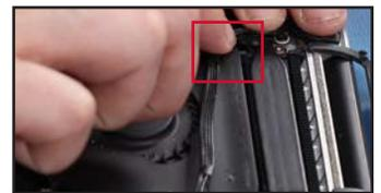
73. Next, lay the cables across the fan and slide the camera cable connector into its socket. Use the nylon pry tool to snap it into place.
