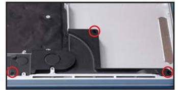
60. Set the logic board back into place, making sure that no cables get trapped underneath it, and that it sits flat.
