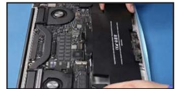
93. Push on the battery board and insert one of the retaining screws in the location shown, then fasten it part way to help align the battery.
