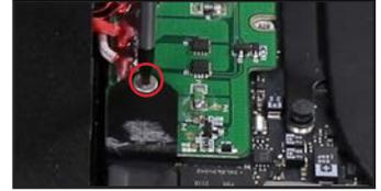
39. Re-affix two Torx T6 screws that you removed in Step 6. Screw locations shown in red.
