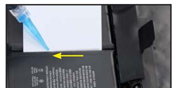
57. Use the card to slice at the adhesive under the battery. You can also use a second card from the other side, but make sure to slice under the battery itself and not under the trackpad that the battery sits on.
