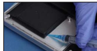
44. Starting at a corner, work one of the plastic cards underneath the battery cell, slicing through the weakened adhesive strips until it detaches. You can use more adhesive remover if you need to, but try and use as little as possible.
