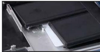
51. Apply a small amount of adhesive remover along the front edge of the battery cells.
