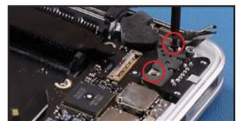
62. Re-affix the longer silver screw near the heat sink and manually reset its rubber cap.
