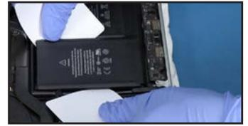
21. Work another plastic card under the remaining cell, repeating the same process. If needed you can use an additional small amount of adhesive remover until the cell detaches.
