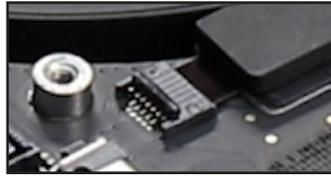
19. Lift the right fan and carefully unstick the cable from the logic board using your fingers, then slide the cable connector out of its socket (right). Now the fan assembly can be removed and set aside.
