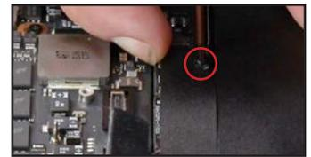
95. Slide the trackpad cable from Step 44 back into its ZIF connector, then latch the connector shut with the nylon pry tool.
