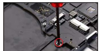
71. Slide the keyboard cable into its ZIF connector until it is fully seated (top row), then lock it into place with the lever on the back. Afterward press the cover down on the connector. It should stick in place.
