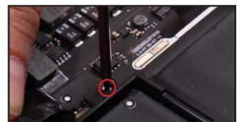
31. Follow the same procedure from Step 30 with the label and screw on the opposite side of the connector.
