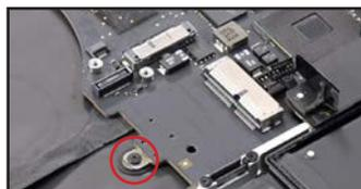
35. Remove the screw near the memory modules.
