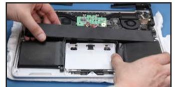
31. Next, re-affix the screws you removed in Steps 13 and 16 to help hold it in place. You may need to adjust the battery's position slightly so that the holes are properly aligned as you affix each screw.
