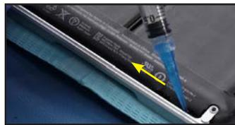
52. Work one of the cards underneath the center cells.
