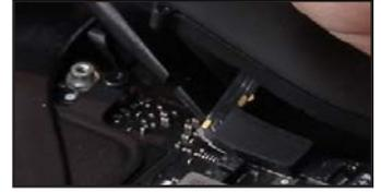
27. Remove the rubber cap (red) from the Torx T5 screw near the heat sink, and then remove the screw itself.
