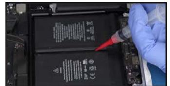
20. Work one of the plastic cards between the center cells, slicing through the adhesive strips until it detaches. You may need to use two cards.
