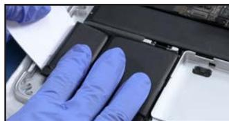
23. Repeat the process on the neighboring cell. Try to use as little adhesive remover as possible.
