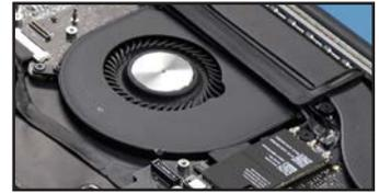
13. Lift the rubber cover off of the right fan and set it out of the way.
