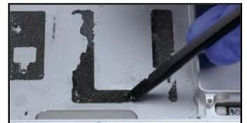
27. Wipe up the extra adhesive remover and let the chassis sit for about half an hour to ensure any liquid has evaporated.
