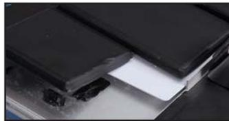
47. Using the syringe apply about a quarter of a milliliter of adhesive remover under the outer battery cell on the opposite side of the computer and let it sit for about a minute.
