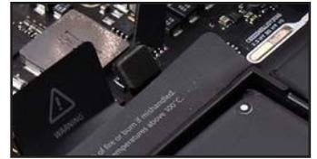
30. Peel back the edge of the label that covers the battery connector and remove the Torx T5 screw near the edge that holds the battery in place.
