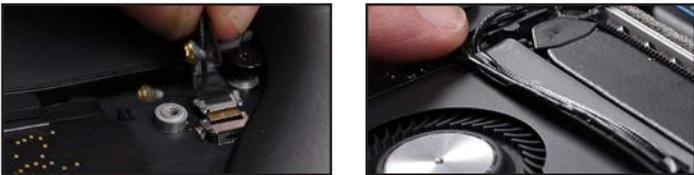
85. Align the wireless card with its socket, slide it into place, and secure it with the screw you removed in Step 15.
