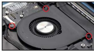
18. Use the nylon pry tool to lift the latch on the fan cable's ZIF connector, shown in red.
