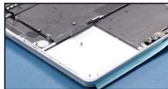
62. Set the right speaker assembly into place, then secure it with the three screws you removed in Step 41.
