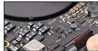
27. Disconnect the left speaker cable using the same method from Step 24.
