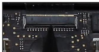
...then, use the nylon probe tool to separate the cable from the battery — enough that you can slide the cable from the connector...
