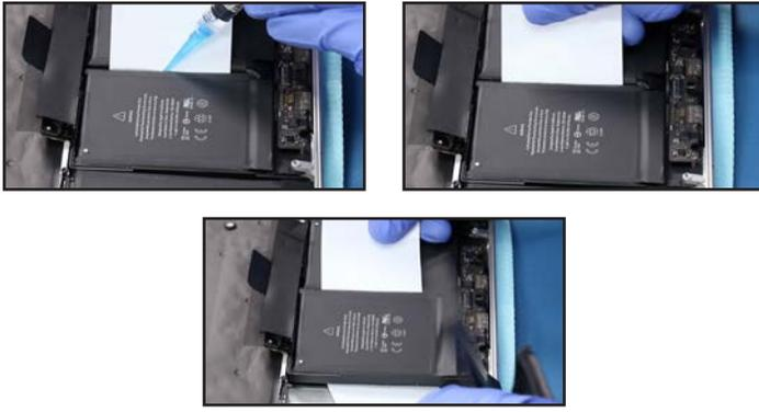
59. Once all the cells have been detached, you should be able to lift the whole battery up and out of the chassis.
