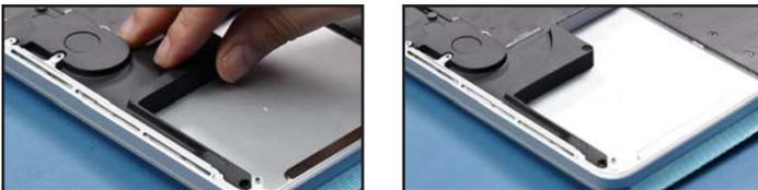
63. Slide the left speaker assembly into place, then secure it with the three screws you removed in Step 43.
