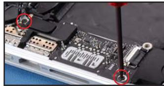
19. Lift the I/O board up and out of the chassis.
