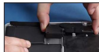
42. Remove the corresponding screws that hold the left speaker assembly in place, then lift it up and out of the macbook pro.
