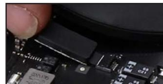
87. Set the fan flat then re-affix the Torx T5 screws that you removed in Step 25, using their original locations.
