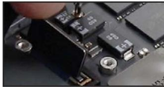
8. Peel back the edge of the label that covers the battery connector (left) and then remove the Torx T5 screw near the edge that holds the battery in place (right).
