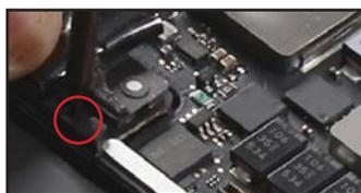
9. Peel back the opposite edge of the same label and remove the corresponding screw.
