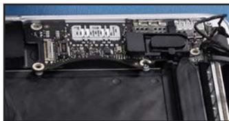
68. Secure the I/O board with its Torx T5 screws, in the locations shown.
