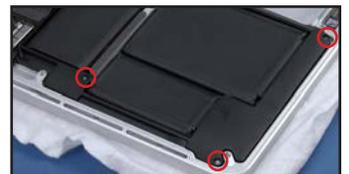
15. Lift the speaker assembly up, and rotate it so that it sits out of the way.
