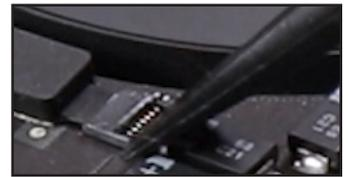
25. Remove the three screws holding the fan in place. Again, each screw is different, so make note of each screw's location. They will have to be re-affixed in the same locations later.
