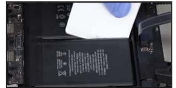
22. Carefully lift the battery unit up and out of the chassis.
