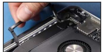
29. Remove the three screws holding the left fan in place. As with the previous fan, note the location of each screw; each is a different length and will need to be re-affixed in the same location.
