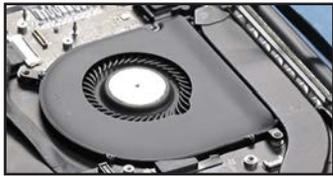
83. Re-affix the three fan assembly screws you removed in Step 17, making sure each is repositioned in its original location.
