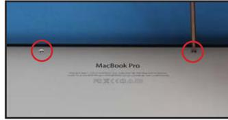
3. Remove the remaining eight pentalobe screws, shown at right.
