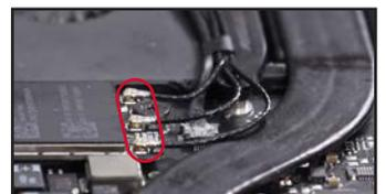
76. Align the SSD card with its socket, slide it into place, and secure it with the SSD mounting screw.
