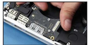
80. Secure it with its two Torx T5 screws that you removed in Step 22.
