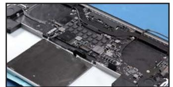
61. Re-affix the two Torx T5 screws that hold the Magsafe connector in place.
