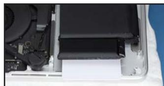
19. For the center cells, use the syringe to apply about a quarter milliliter of adhesive remover between the two cells and let it sit for about a minute.
