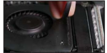
13. Remove the three Torx T5 screws affixed to the fan housing. Note the location of each screw before setting them aside; each is a different length and will need to be re-affixed in the same location later.
