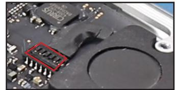
28. Lift the rubber cover off of the left fan and set it back and out of the way.
