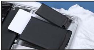
21. Using the syringe, apply about a quarter of a milliliter of adhesive remover under the outer battery cell on the opposite side of the computer; let it sit for about a minute.
