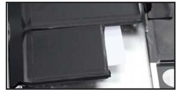
55. For the center two cells, first slide a card in between the batteries, so that it starts to lift one of the cells.
