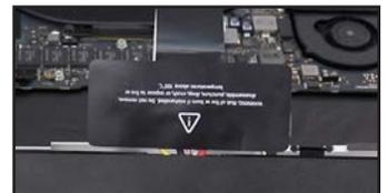
29. Peel off the paper backing covering the adhesive on each side of the battery.
