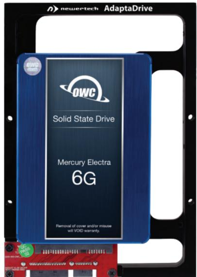
The NewerTech AdaptaDrive can be installed into your computer's 3.5-inch SATA drive bays as well. The example below shows the AdaptaDrive being installed into a Mac Pro.
