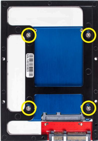
3. There are eight Phillips head screws included. Use the four fine-threaded screws to fasten the AdaptaDrive to the SATA drive.
