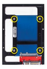
There are eight Phillips head screws included. Use the four fine-threaded screws to fasten the AdaptaDrive to the SATA drive.
