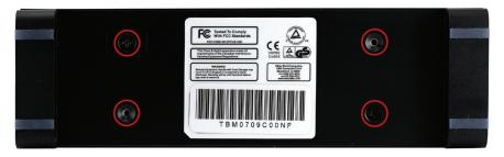
Turn the drive enclosure onto it's side as shown and remove the Phillips screws that are inserted into the bottom of the drive enclosure. This will release the internal drive carrier. Slide the drive carrier out of the external housing, pushing it to the front.
