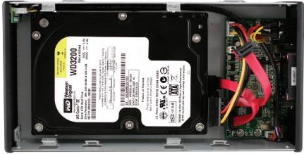
Important note: You must use identical size and model hard drives in this enclosure - you may NOT use 2 different size, or model mechanisms.
