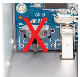
Do not unplug any of the cables on the logic board of the NewerTech Guardian MAXimus drive enclosure.
