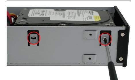
Insert 4 Phillips screws into the top hard drive, fully securign it into the NewerTech Guardian MAXimus drive enclosure. There are 2 screws on each side of the enclosure. Make sure to tightend them securely.
