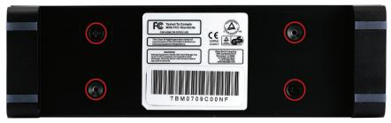
Turn the unit on it's side and insert the 4 Phillips screws to secure the enclosure to the outer shell.
