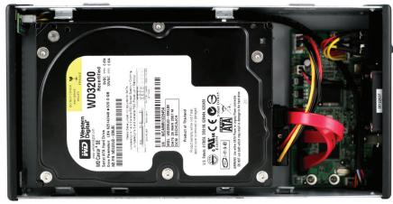
Turn the hard drive enclosure back over and insert the top identical model hard drive. Insert the power and SATA cables into it, as you did with the bottom drive.
