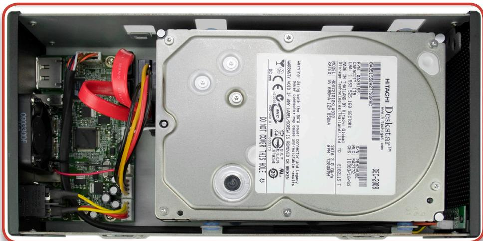
Gently set the 2nd hard drive on top of the lower drive that's already installed into the chassis and once again, plug in the multicolored power cable and red SATA cable into the drive. This drive is easier to install.
