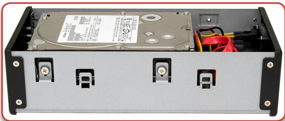
Once the cables are installed, look at the side of the drive chassis and align the screw holes in the sides of the hard drives up and fasten the same collared screws that you used on the bottom drive through the silicone rubber grommets and attach one side of the hard drive into the chassis. Repeat on the opposite side of the chassis.
