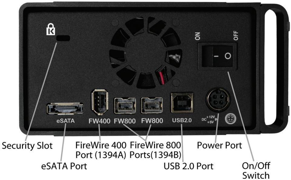
Turn the Newer Technology Guardian MAXimus so you can see the rear port as shown above. First, make sure that the power switch is off. Then, connect the power cable to the back of the Guardian MAXimus. Finally, you need choose which interface you want to use to connect to your computer.
