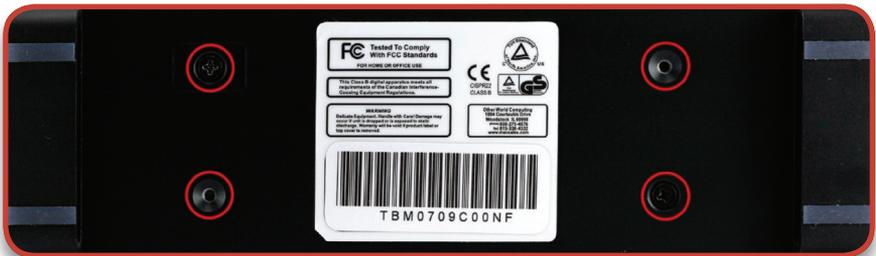
Again, lay the Newer Technology Guardian MAXimus onto it's side and insert the 4 black Phillips screws (2 you removed to start this process, and 2 from the bag) through the outer shell into the inner chassis, fully fastening the Newer Technology Guardian MAXimus together and completing the assembly process.
