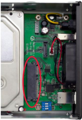
4. Install the first hard drive (HDD1), as shown to the left. Slide the SATA connector on the hard drive into the black SATA connector circled in red. Make sure the drive is firmly seated in the black SATA connector before proceeding.
