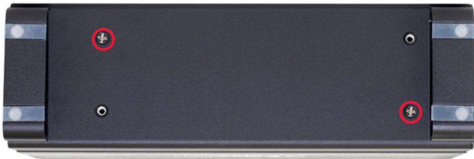
2. Once the two screws have been removed, slide the inner chassis out of the front of the outer enclosure, as shown below. Start by pushing on the rear of the inner chassis, then when you are able to get a grip on the front grill of the inner chassis, pull it the rest of the way.
