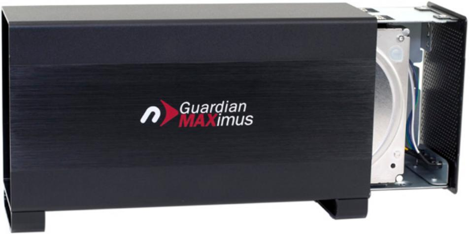
9. Once the front grill of the inner chassis sits flush with the edge of the outer enclosure, turn the Guardian MAXimus on its side again to look at the screw holes on the bottom. You should see that the screw holes in the outer enclosure line up with the screw holes in the inner chassis. Use the four smaller screws to fasten the inner chassis to the outer enclosure, as shown below. The assembly of the Guardian MAXimus is now complete.
