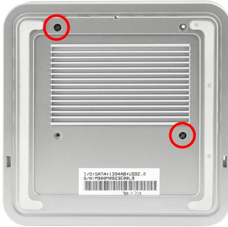
Remove the miniStack housing from its protective plastic bag and turn it over so you can see the bottom of the enclosure. There are 2 Phillips screws securing the aluminum ribbed heatsink into the enclosure for transport. Remove the 2 Phillips screws and take the heatsink out of the enclosure.
