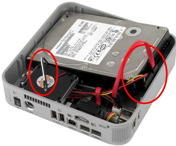
Insert your hard drive into the miniStack v3 enclosure, front first, as shown in the photograph. Pivot the hard drive up so you have access to the SATA power and SATA data cable ports, and plug the SATA power and SATA data cables into the drive. Also, make sure that the white and black thermal probe cable is not pinched but accessible as shown. You will want to orient it so that it comes out the left side of the fan.
