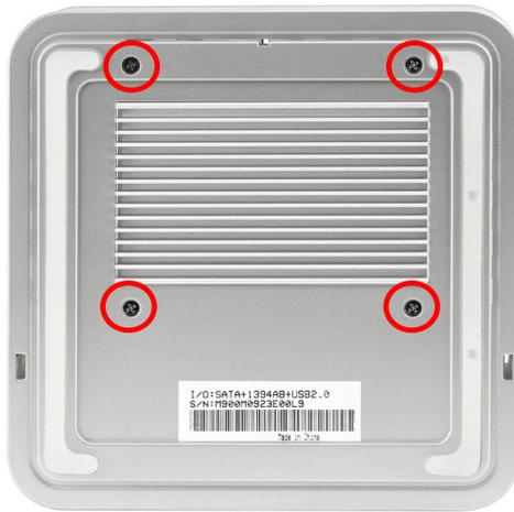
Pick up the miniStack v3 and while holding the hard drive down into the enclosure fully, take the 2 Phillips screws you initially removed from the heatsink and reinsert them into the heatsink through the bottom of the enclosure. Then, remove two more screws from the plastic bag and insert those through the remaining two holes to fully secure the heatsink into the miniStack v3 enclosure.
