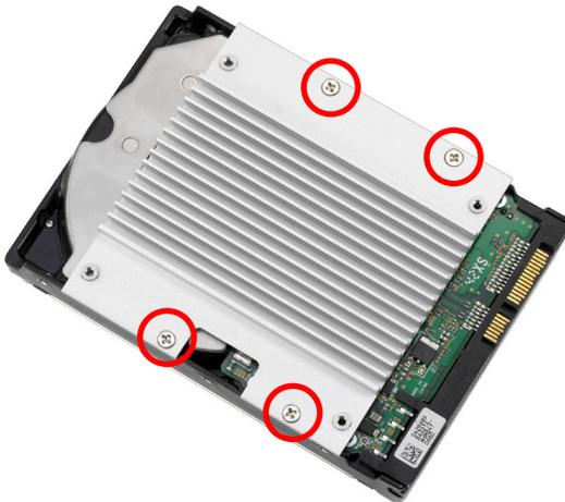
Take your hard drive mechanism and place the aluminum heatsink on the drive as shown. Make sure to orient the cutout notch exactly as shown, to the left, when looking from the back of the drive. Using the 4 Phillips coarse thread screws from the plastic bag, firmly affix the heatsink to the drive.
