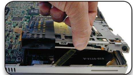
*Be careful to note the positioning of the grommets that are located near the four corners of the drive. They allow the drive to align with the slot in the frame, so that discs may be inserted and ejected smoothly.*
