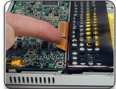
You should be able to detach it by simply lifting up on it with your finger nail.
