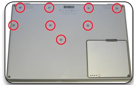
Once the screws are out, you should be able to remove the bottom cover. It is recommended to start loosening at the corner where the battery sits.
