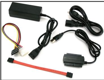
To begin, remove the contents of the shipping box and lay them out in front of you. You will see that there is a Universal Drive Adapter, a power supply, a power cable, a Serial ATA cable, and a Serial ATA power adapter cable.
