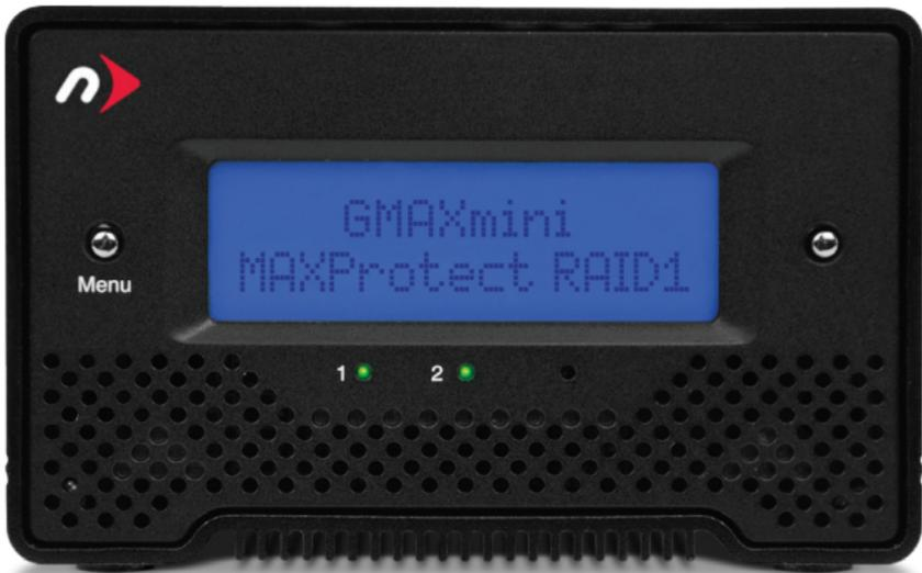
The Newer Technology Guardian MAXimus mini has an LCD display at the front of the hard drive enclosure. It will illuminate blue when powered on, and the activity lights below the LCD display will also illuminate. The LCD display is covered in more detail in the next pages.
