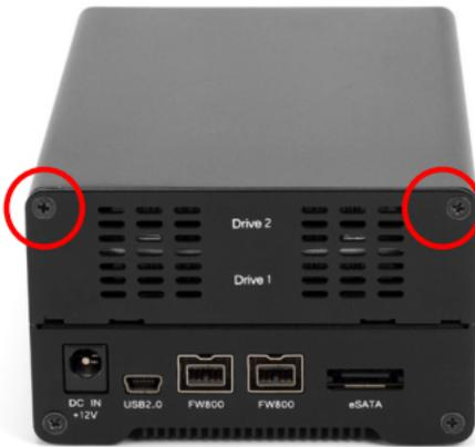
To remove the drives, turn the Newer Technology Guardian MAXimus mini around to the rear and remove the hard drive cover plate by unscrewing the 2 Phillips screws from the top corners.
