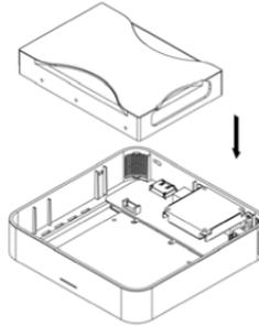
3. Turn the enclosure around and fasten the four screws.
