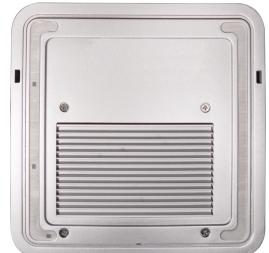
carrier from inside of the Newer Technology miniStack enclosure. the Newer Technology miniStack enclosure. Remove the drive I. Begin by removing the 4 Phillips screws from the bottom of
