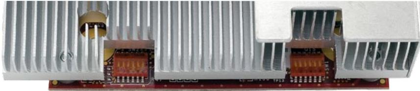
All Newer Technology MaxPower G4 upgrade cards are shipped preconfigured from the factory to use with 133MHz Power Macintosh systems right out of the box. If you have a 100MHz Power Macintosh G4 AGP "Sawtooth" or "Gigabit Ethernet" system, you need to adjust switches to properly work with your system.
