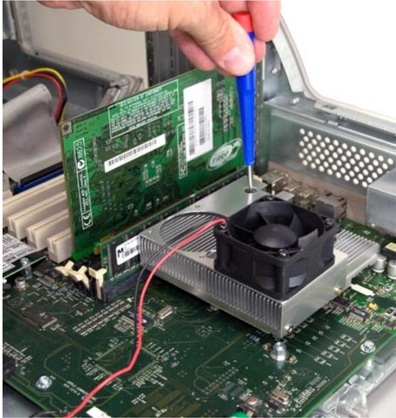
• Using the original screws, secure the Newer Technology MAXPower G4 card into place on the motherboard. This is a little tricky as the screws have to be placed through the heatsink.
