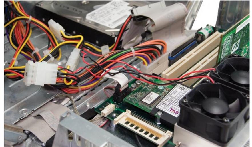
Connect the 4 pin wiring harness for the fans to one of the disk drive power connectors. A pass thru connector is provided.
