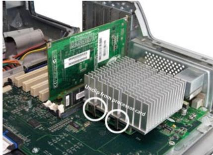
• Review the static-safe procedures from Page 4 before proceeding. Open the case of your Power Macintosh and look at the processor card. There were a couple of different heatsink configurations shipped in this model of computer, yours may have a plastic shroud and fan assembly attached to it. If so, unclip the plastic shroud, and unhook the fan wire from the processor card, it pulls straight out. In all configurations, proceed to the heatsink clip removal.
