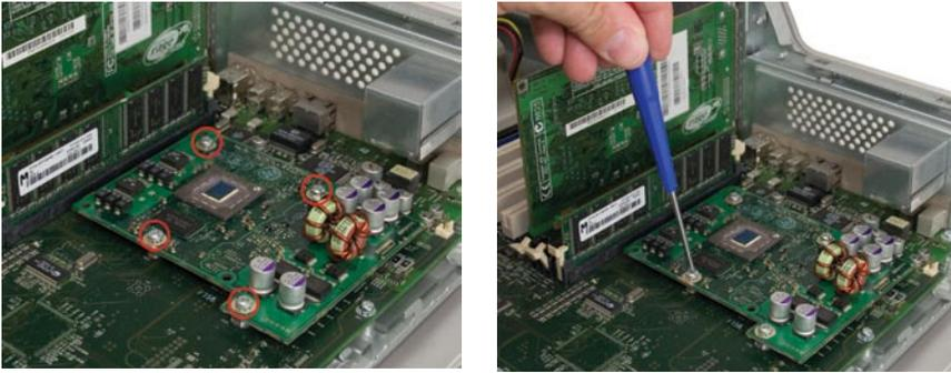
• Remove the screws that hold the Apple CPU card in place. Be careful not to lose the screws as you will be reusing 3 of the 4 of them to install the Newer Technology MAXPower G4 processor upgrade card.
