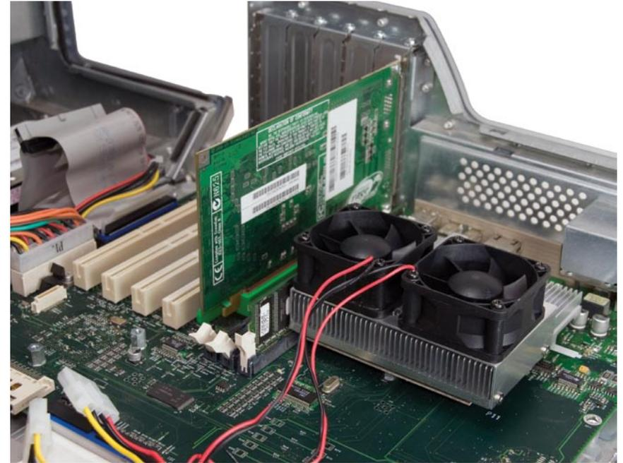
• Once the processor card is screwed into the logic board, set the included 2nd fan onto the heatsink, as shown. Make certain that the wires are next to the fan that is already attached to the heatsink. Screw the 4 Phillips screws at the corners of the fan into the heatsink.
