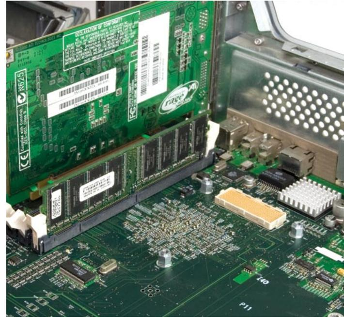
• Carefully pull the original processor card straight up and out of the motherboard socket. Remove the protective cap (with the neon green sticker) from the socket on the Newer Technology MAXPower G4. (See picture below.) Place the cap on your original Apple CPU card.
