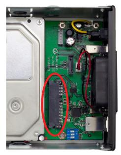
Insert your first drive into the chassis of the Newer Technology Guardian MAXimus. Place the rear of the drive (the end with the SATA and power connection) onto the green bridge board as shown.
