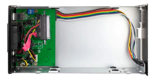
Once you have removed the inner chassis, look into the chassis you will also see the cables, and screw holes that you will be using in future steps.
