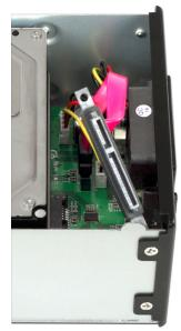
Reach in behind the hard drive and manipulate the combination SATA data and SATA power cable around so that the long L shaped opening in the cable is oriented in the same position as you see in this photograph.
