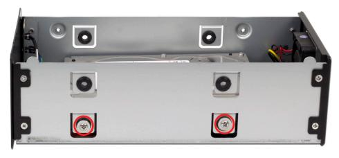
Using 4 of the large screws that were in the clear packet you removed from the chassis of the Newer Technology Guardian MAXimus, fasten the hard drive to the chassis using the lower screw holes.
