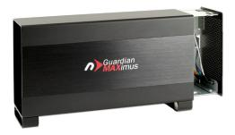
Turn the Newer Technology Guardian MAXimus onto it's side and remove the 2 scews that are fastening the outer shell to the inner chassis.
