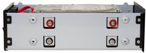
Place the second hard drive into the enclosure and line up the screw holes on the side of the chassis.
