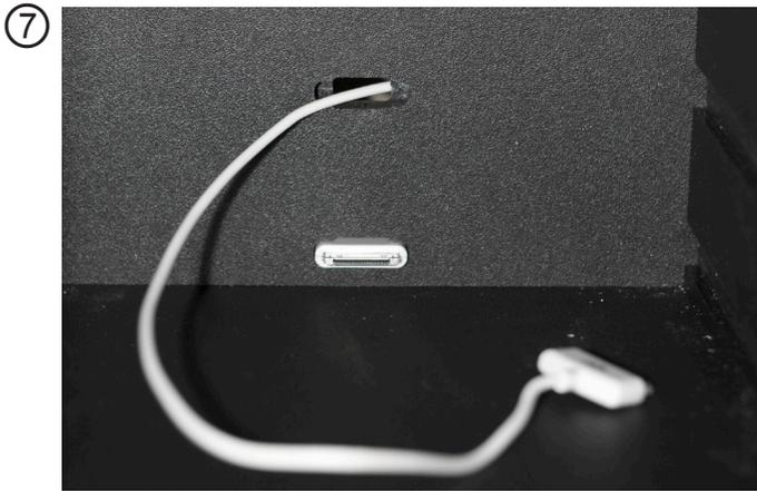
Once you have released the dock cable from the GripStand Station, remove it from the black wire loom that is used for cable management. Then, slide the cable out from the inside and remove it completely.
