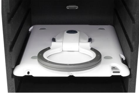
Once the iPad reaches the back of the GripStand Station, you will feel slight resistance and may even hear a “click” as the iPad connects with the 30-pin dock connector. The GripStand Station is designed to prevent damage to the iPad’s dock connector by distributing the insertion force across the surface of the GripStand case, not the iPad itself. Gentle pressure is all that is needed to insert the iPad into the GripStand Station.
