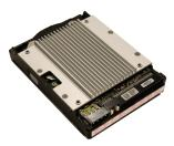
**2.** Make certain that the hard drive mechanism you're installing inside the Newer Technology miniStack v2 enclosure is set to MASTER before installing. You can find this information either on the drive mechanism, or by visiting the drive manufacturer's website.
