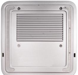
**1.** Begin by removing the 4 Phillips screws from the bottom of the Newer Technology miniStack v2 enclosure. Remove the drive carrier from inside of the Newer Technology miniStack v2 enclosure.
