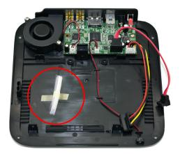
Turn the miniStack over and place the bottom on the work surface. Lift the top cover off of the miniStack, exposing the internal chassis.
