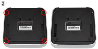
Turn the Newer Technology miniStack over placing the top on a soft work surface, such as a towel.
