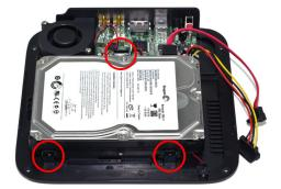
Place your drive into the chassis of the miniStack. There are 2 rubber coated mounting tabs with screwholes on the side closest to you in this photograph, and a tab with a plastic detent on it that will lock the drive into the chassis on the center of the drive on the opposite side. You will need to set the drive into this detent in the tab to insert the drive.
