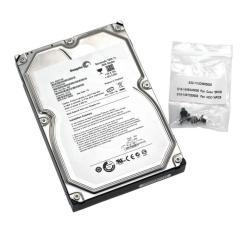
Make sure that the hard drive you wish to install (sold separately) is handy and remove the screws from the bag.
