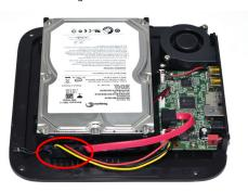
Turn the enclosure so that the side of the hard drive with the connecting ports are visible. Insert the SATA and power cables into the hard drive. They are keyed to only go in one direction.
