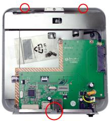
Lift the top cover off of the bottom enclosure of the miniStack Classic. This can be a bit challenging, as there are a number of concealed clips that help secure the top cover onto the bottom enclosure.
