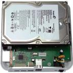
Place your drive into the chassis of the miniStack Classic. There are 2 mounting tabs with screwholes on the side furthest away from you in this photograph, and one screw post on the side closest to you.
