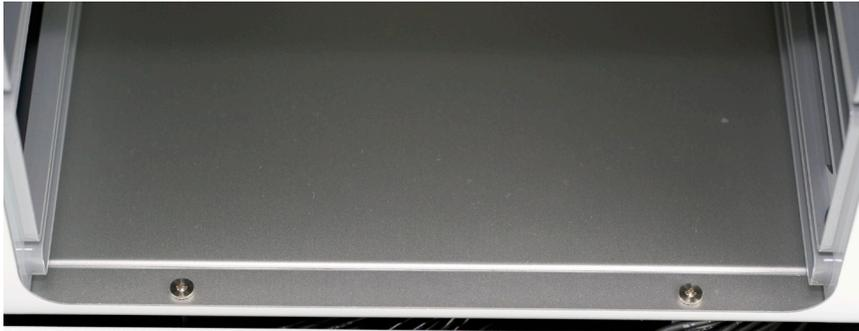
At the bottom of the memory bay, there are 2 more Phillips screws. They are a smaller head than the ones inside the memory bay that you just removed. Use a Phillips #0 screwdriver to remove the screws.
