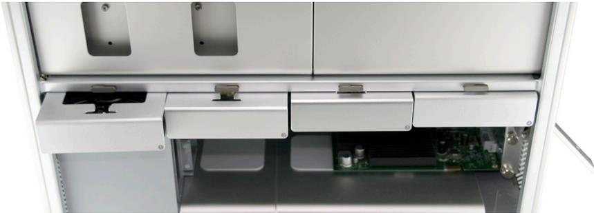
Make sure that the locking latch on the back right side of the Mac Pro. Then, remove all 4 of the drive bays and set them aside.
