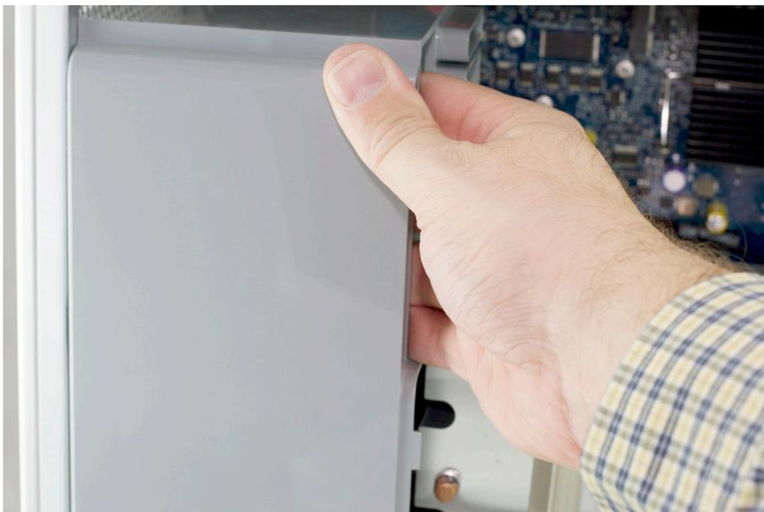
Using your right hand, wiggle, tug, and pull the entire fan assembly out of the computer. It attaches to the logic board via a connector that you don't need to worry about disconnecting, it's a pressure fit.
