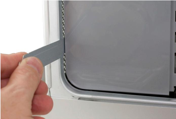
Take the L shaped PCI card deadplate you removed on page #7. Starting at the top of the fan shroud, work the short end of the bracket into the gap at the back of the Mac Pro, as shown above.
