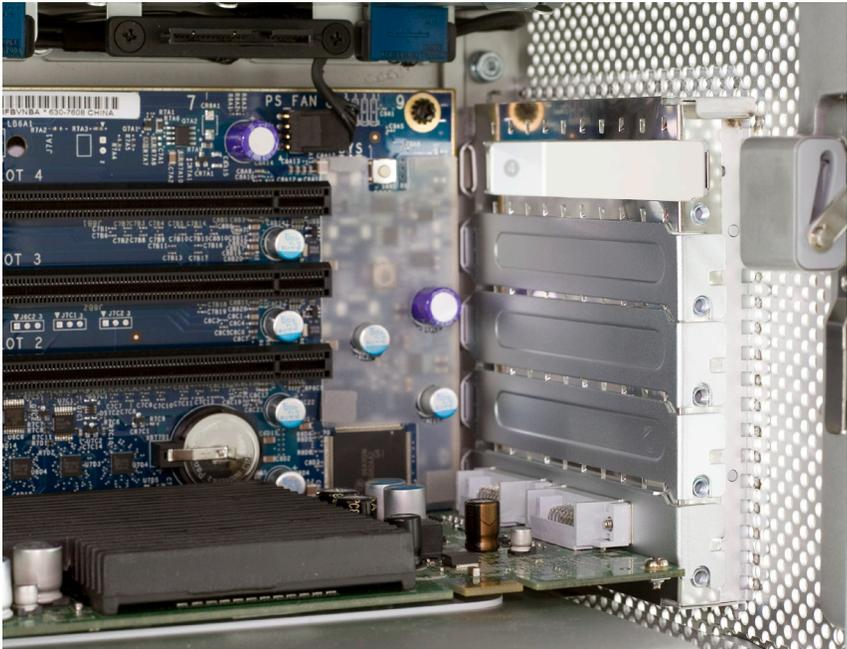
Once the metal retaining plate is removed, remove the top PCI Express dead plate cover from the top slot as shown. Set the dead plate cover aside, you'll be using it in a future step.
