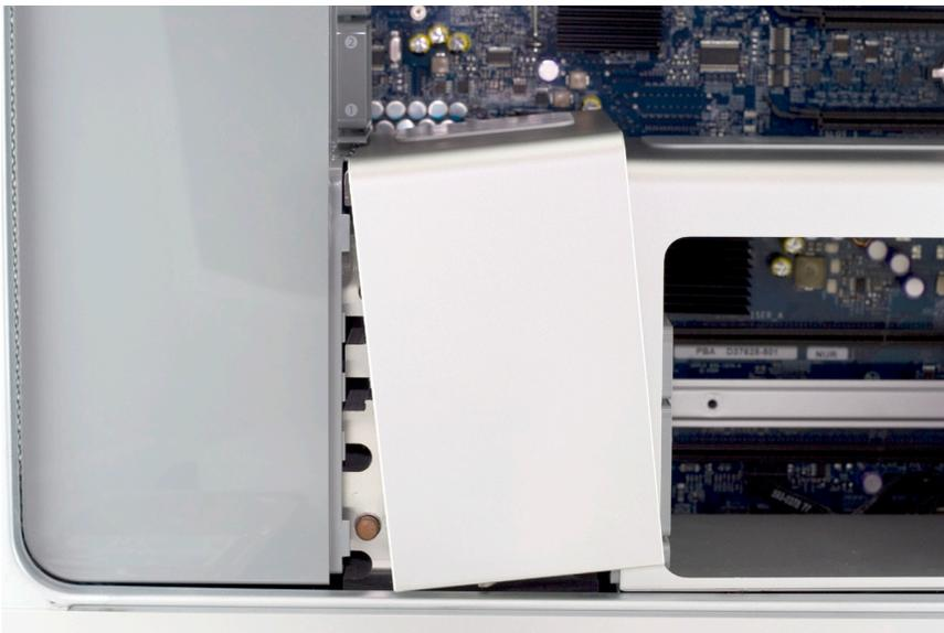
Once the memory bay is moved, you can pull out on the bottom of the processor cover on the bottom right, and gently remove it from the computer. It hinges up and to the right as shown. It locks into the fan shroud on the left fairly tight.
