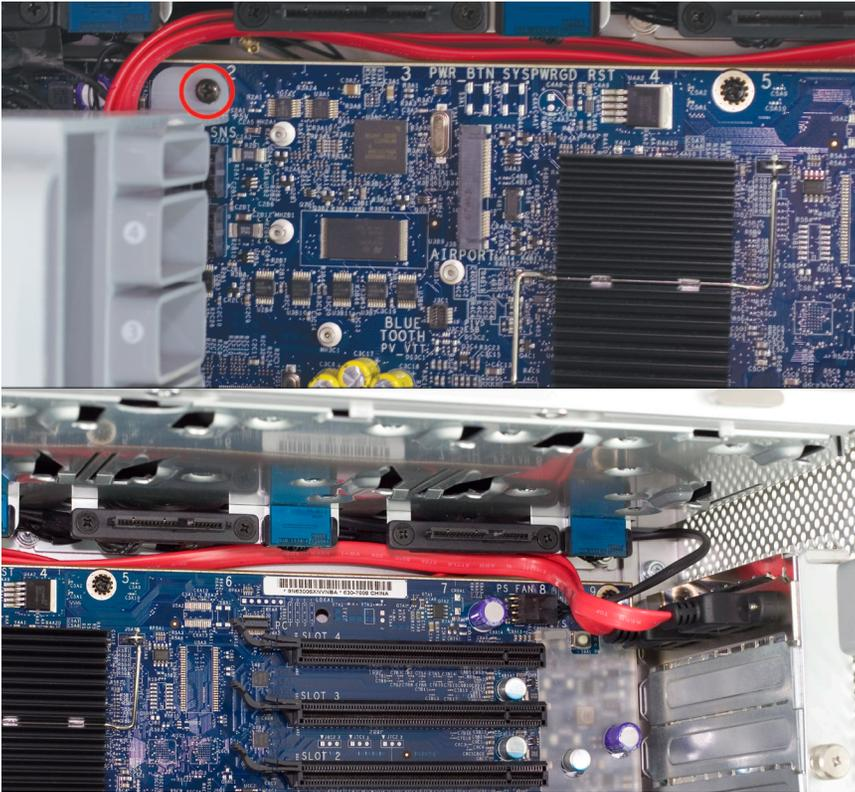
Here are 2 pictures of the Mac Pro Quad Xeon eSATA Extender Cable completely installed. Finish routing the SATA cables and double check that you have them completely behind the rectangular black SATA drive connectors at the top of the Mac Pro.
