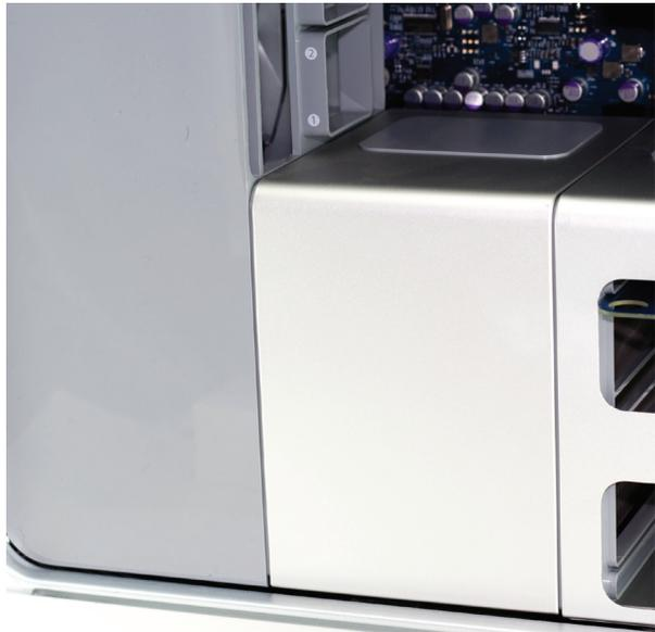
Remove the cover over the processors by pulling on it. There are magnets securing the cover in place.
