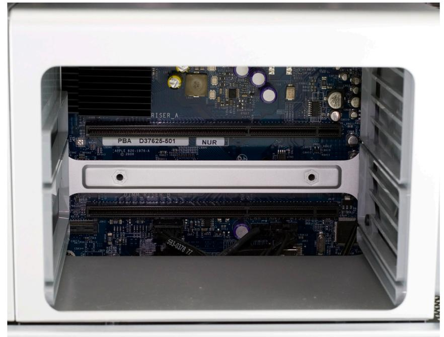
Remove the 2 Phillips screws. They are long and extend through the logic board and into the back of the computer.
