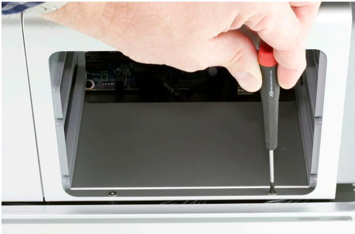
A photo of this task being made look easy, at least if your screws are not improperly installed as described above. Try and not strip the Phillips screw heads.
