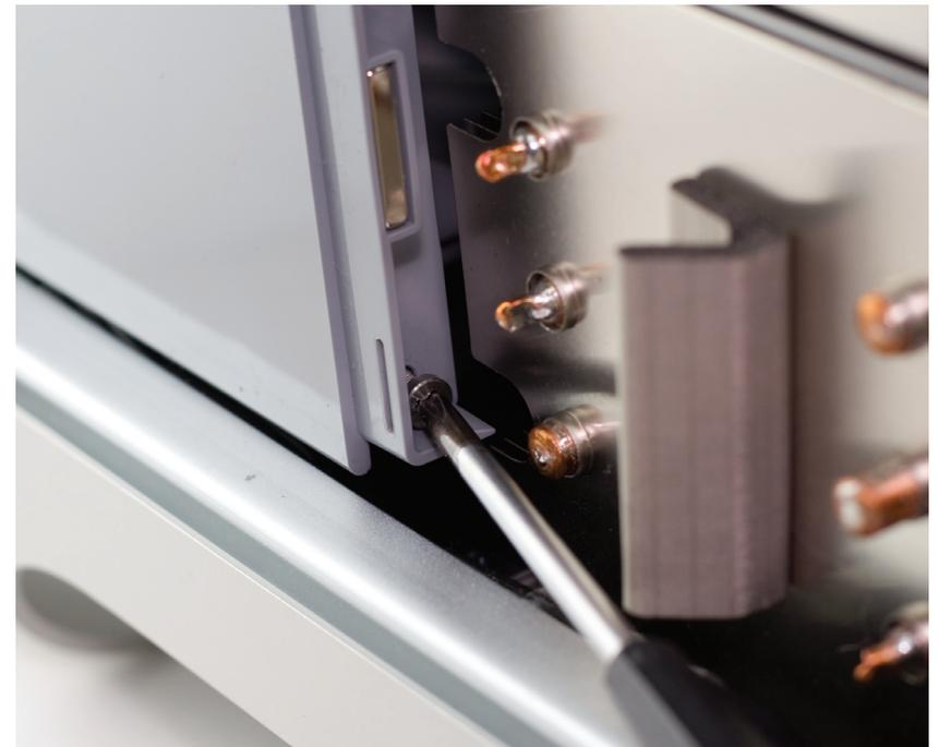
Some later model Mac Pro systems, especially 8-Core models, have a hidden Phillips screw located at the base of the fan assembly. Unscrew it.
