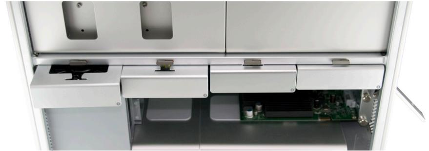
Make sure that the locking latch on the back right side of the Mac Pro. Then, remove all 4 of the drive bays and set them aside.
