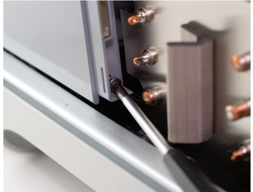
Remove the Phillips screw from the base of the fan assembly, located at the bottom left of the processor heatsinks.
