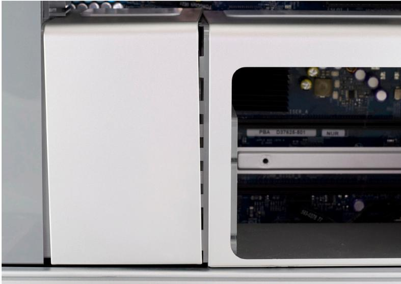
Take the memory bay and gently move it to the right, towards the back of the computer. You'll be able to gently shake it and it will pop loose and move just enough to expose a gap between the processor cover and the memory bay as shown.
