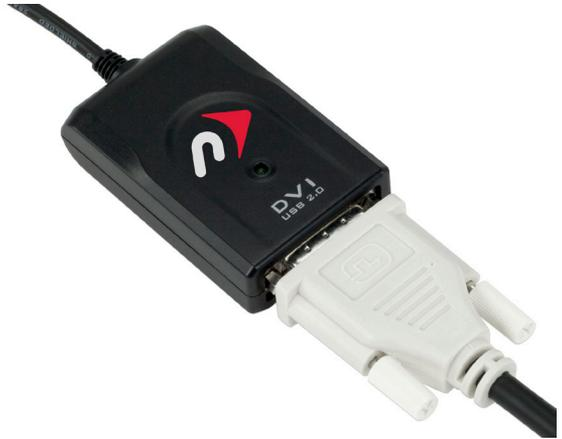
**Step 2.** Connect your NewerTech USB to DVI/HDMI/VGA Video Display Adapter to your computer using the USB 2.0 "A" cable
